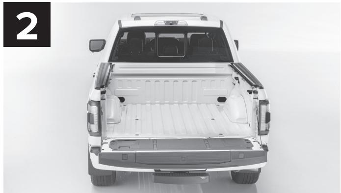
Remove ImpactLiner from the shipping box and unroll on a flat, dry surface. DO NOT install if the temperature, or your truck bed, is below 50° F.
