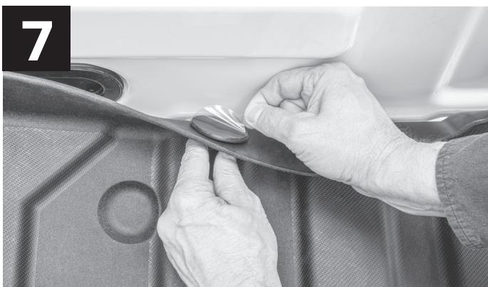
Remove the plastic backing from each TechHold Ball and lay ImpactLiner down while pressing the TechHold Ball against the truck bed wall. Hold for a minimum of 15 seconds to adhere disc. Ensure both are adhered prior to step 9.
