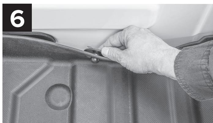
Place ImpactLiner into the truck bed and locate two previously trimmed holes on the front of the ImpactLiner. Use cloth to clean the area behind the trimmed holes with mild soap and water. Allow to dry. Use the supplied alcohol wipe to prep the truck bed wall surface for the TechHold Ball and Socket Retention Devices.
