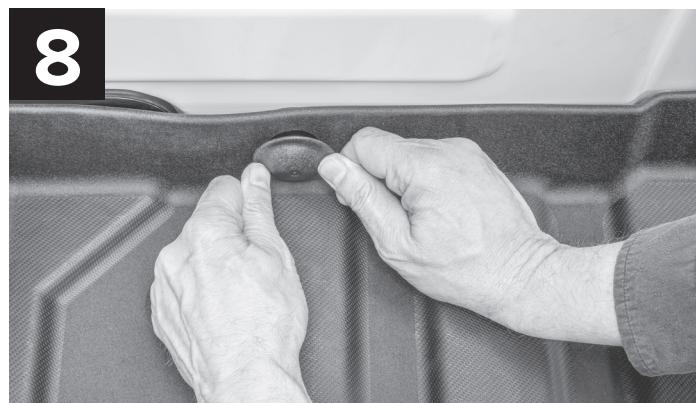
Once both TechHold Ball Devices are properly adhered, lay ImpactLiner over them, so the TechHold Ball Device passes through the two trimmed rings. Take the TechHold Socket and press onto TechHold Ball Device until an audible click is heard. ImpactLiner is now secured.
