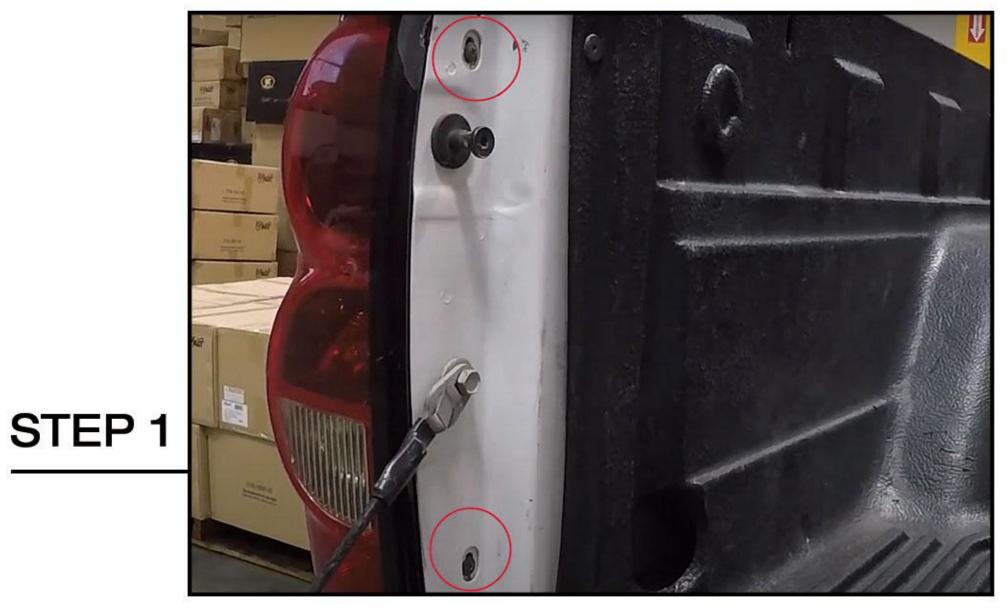
Remove Two screws on the top and bottom.
