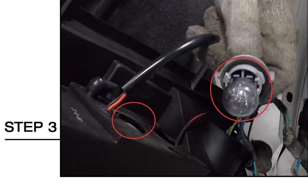
Plug this silver socket bulb directly into the new taillight.
