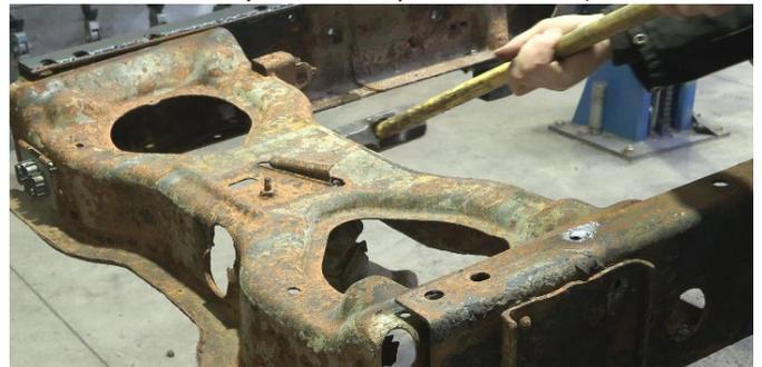
Grind the work area free of rust and debris, revealing bare metal, followed by coating the work area with a weld through primer to help prevent against further rust development.
