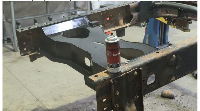
Insert the included hardware and secure the sections and hangers with a 14mm socket and 15mm wrench.
