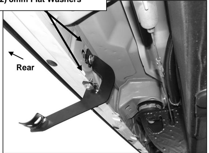
(Fig 6) Driver side 3rd mounting location pictured
