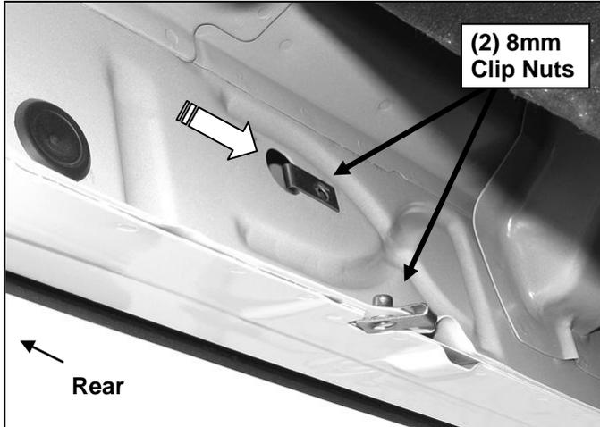
(Fig 5) Driver side rear mounting location pictured
