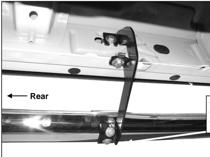
(Fig 7) Driver side 3rd mounting location pictured
