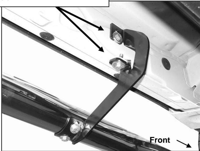
(Fig 3) Driver side front mounting location pictured
