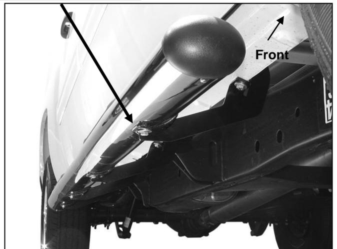
(Fig 8) Passenger side front mounting location pictured
