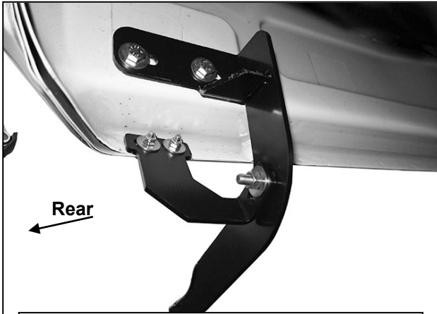
(Fig 16) Driver/Left rear Brackets installed
