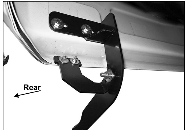
(Fig 14) Driver/Left rear Brackets installed
