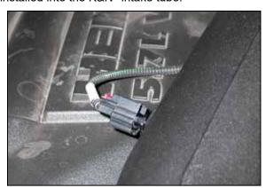
27. Connect the provided inlet temperature sensor extension into the factory wiring harness and then connect the other end to the inlet temperature sensor.
