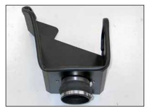
14. Install the silicone hump hose (08418) onto the filter adapter and secure with the provided hose clamp.
