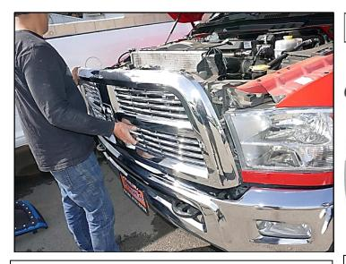
Step 3 Firmly grab and pull factory grille off vehicle. Discard factory grille.
