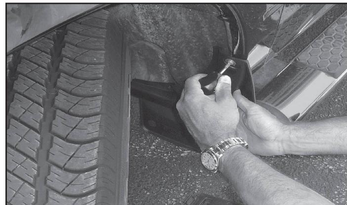
**8** While pressing the MudFlap firmly against the fender, tighten the (2) fasteners.
