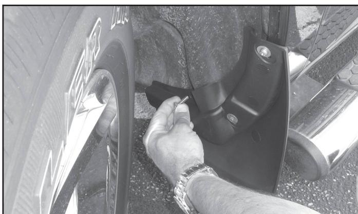
**9** (Optional) For additional support, a  $\frac{1}{4}$ " hole can be drilled or cut into the plastic liner behind the 3<sup>rd</sup> hole provided in the MudFlap. Once the (2) fasteners have been tightened, use the 3<sup>rd</sup> hole in the MudFlap as the guide to drill an additional hole (this hole will only be in the plastic). Use provided hardware.
