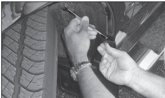
**7** **Small Chip Guard Only:** Using the box end wrench, hold the nut for the smaller machine screw behind the hole in the fender. Attach the machine screw with washer through the MudFlap. (Large Chip Guard only skip to Step 8.)
