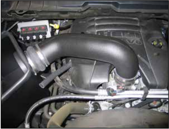
25. Install the K&N intake tube into the silicone hump hose and then into the silicone hose at the throttle body. Align the heat shield assembly for proper fit and then tighten the heat shield mounting bolts then tighten the hose clamps securing the intake tube.
