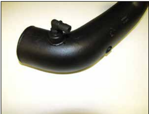
22. Install the 1/4npt vent fitting into the K&N intake tube as shown.
