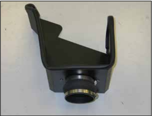
14. Install the silicone hump hose (08418) onto the filter adapter and secure with the provided hose clamp.
