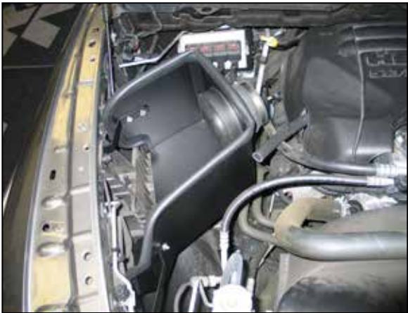
19. Install the heat shield assembly into the vehicle and secure with the bolts removed in steps #17 and 18. Do not completely tighten at this time.
