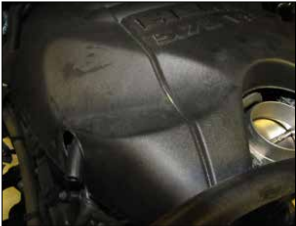
10. Reinstall the engine cover and position the CCV hose through the opening.
