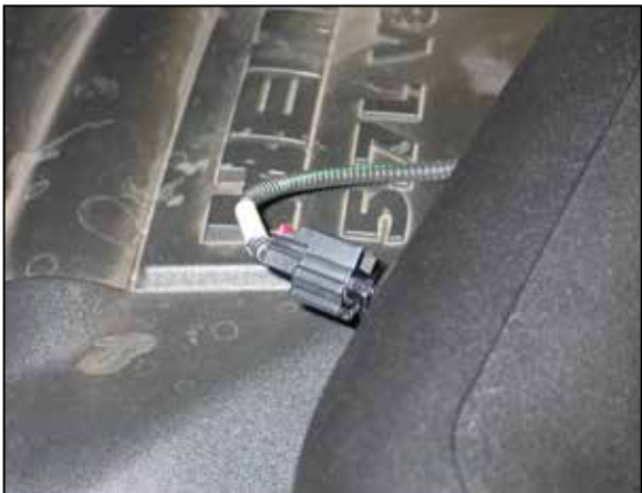
27. Connect the provided inlet temperature sensor extension into the factory wiring harness and then connect the other end to the inlet temperature sensor.
