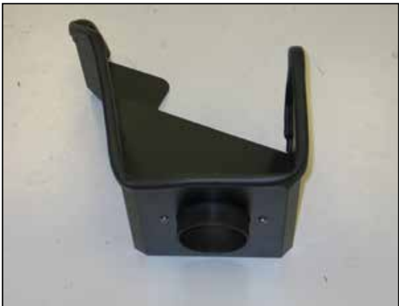
13. Install the provided filter adapter onto the heat shield as shown and secure with the provided hardware.
