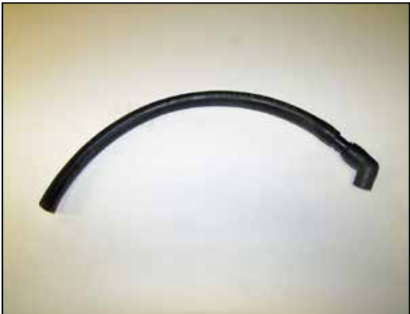
8. Remove the factory 45 deg. elbow from the factory ccv hose assembly. Assemble the K&N CCV hose, union and factory 45deg. elbow as shown.
