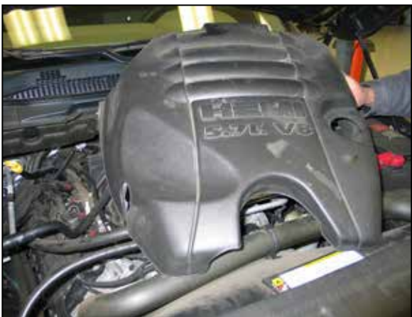
6. Lift up the engine cover to dislodge it from the mounting posts and then remove it from the vehicle.
