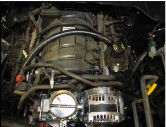
9. Install the K&N CCV hose assembly onto the factory port and position the assembly as shown.
