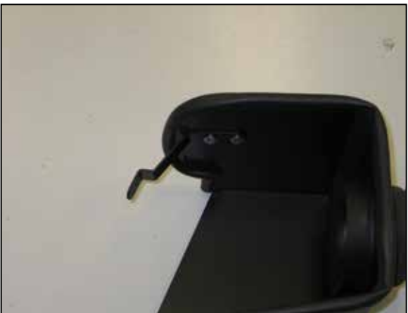
15. Install the heat shield mounting bracket (083127) onto the heat shield using the provided hardware. NOTE: Do not completely tighten at this time.
