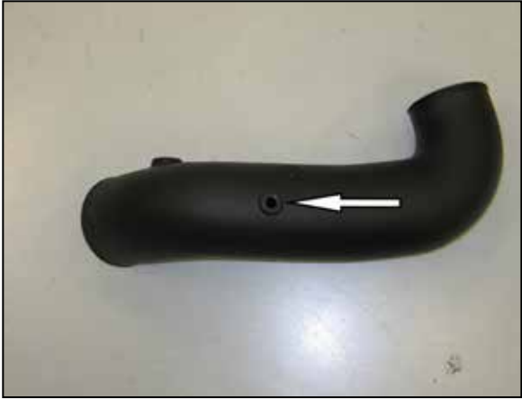
21. Install the provided grommet into the K&N intake tube as shown.
