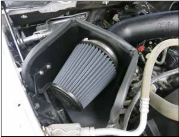
28. Install the K&N air filter and secure with the provided hose clamp.
