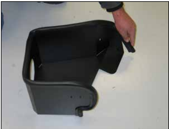
12. Install the provided edge trim onto the heat shield as shown. NOTE: Some trimming of the edge trim will be necessary.
