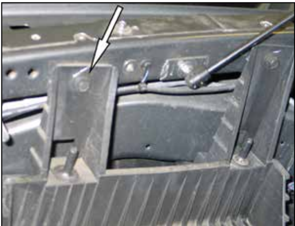
17. Remove the front air box mounting bracket bolt shown. NOTE: This bolt will be used in a later step.
