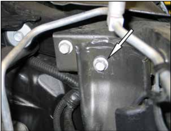
18. Remove the front fender mounting bolt shown. NOTE: This bolt will be used in a later step.
