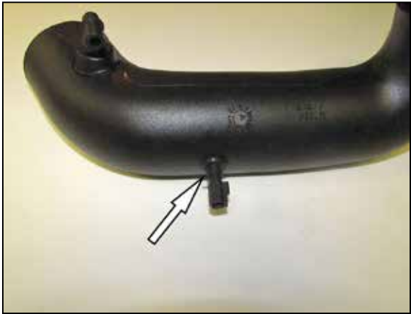
24. Install the inlet air temperature sensor into the grommet installed into the K&N intake tube as shown. NOTE: Take care while installing the inlet air temperature sensor as it is very fragile.
