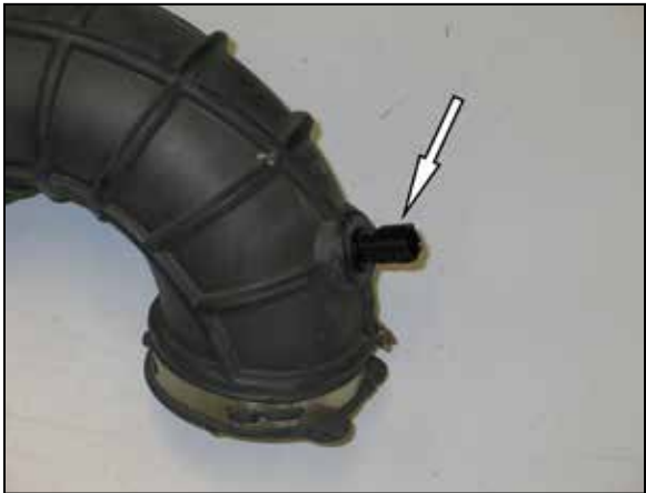
23. Remove the inlet air temperature sensor from the stock intake tube. NOTE: Take care removing the sensor as it is very fragile.
