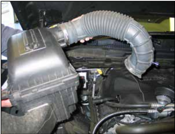
5. Disconnect the factory intake hose from the throttle body, then lift up the air box assembly and then remove it from the vehicle.
