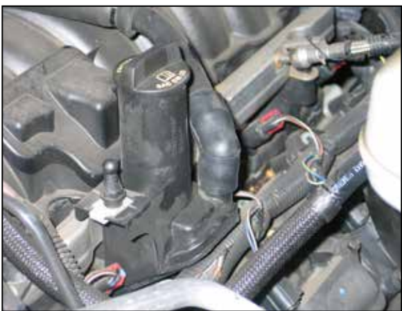
7. Disconnect the crank case vent hose from the valve cover port.
