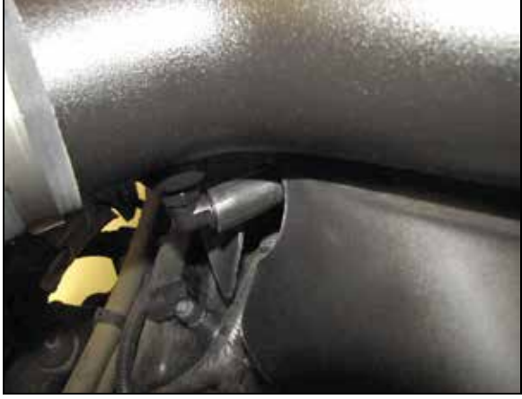
26. Connect the crank case vent hose to the vent fitting installed into the K&N intake tube. Secure with the provided tie wrap. NOTE: Some trimming of the vent hose will be necessary.
