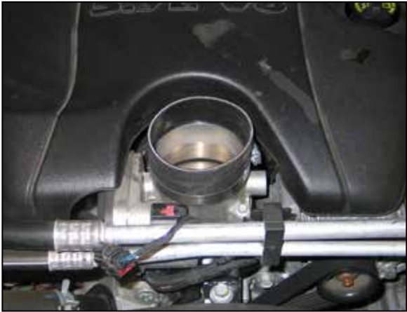
20. Install the provided silicone hose (08698) onto the throttle body and secure with the provided hose clamp.
