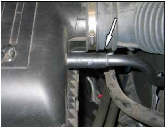
4. Disconnect the crank case vent hose from the air box.
