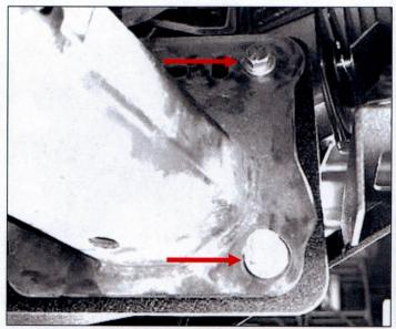
Step 2. With help from assistance place bumper onto the vehicle. Secure bumper onto vehicle using the supplied M12 nut plat, M12 bolts, M12 washer, & M12 hex head nuts. Repeat step for other side.
