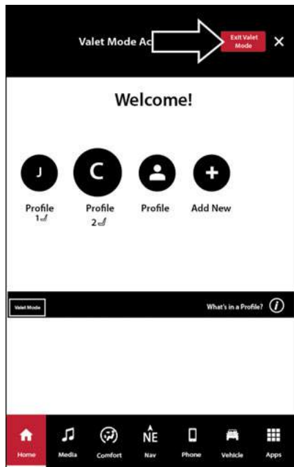
Uconnect 5 NAV With 12-inch Display Or 14.5-inch Display (Portrait) Exit Valet Mode
