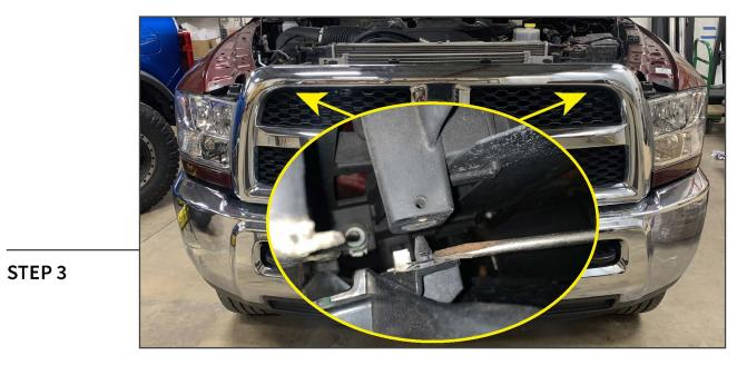
Using a flathead screwdriver, gently pry/twist to dislodge the (2) upper grille retaining clips.
