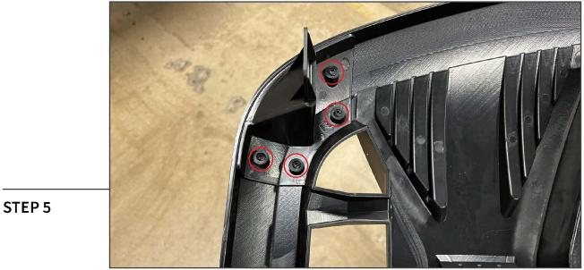
Secure each appropriate upper corner mounts using (4) Phillips screws per mount.
