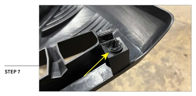
Install the (2) included retaining clips into the lower brackets.
