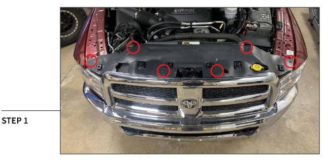
Open the vehicle hood. Remove (6) plastic push clips from the upper radiator cover.
