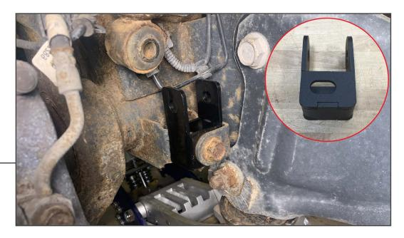
Mount the shock absorber mounting bracket to the shock absorber axle mount using the OEM bolt and flag nut.
