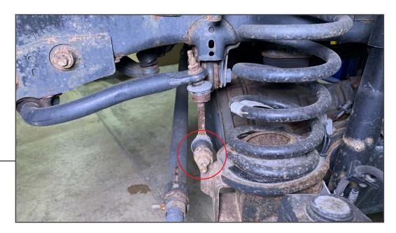
Remove (1) 21mm nut to disconnect the sway bar link from the axle.
