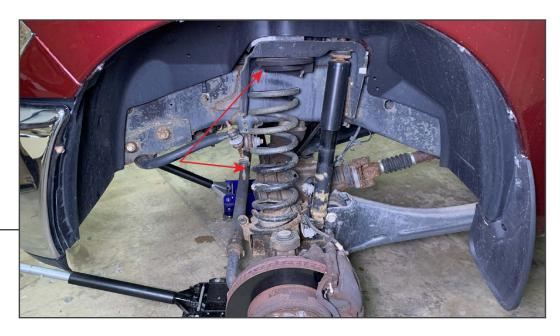
Lower the floor jack slowly to relieve tension from the coil springs. Remove the coil springs and the upper spring isolators from the vehicle.
