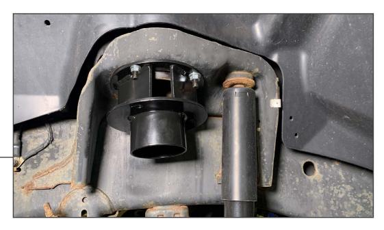
Once drilled, re-mount the upper spring spacer using (2) M10 x 30mm bolts, (2) M10 flat washers, and (2) M10 nuts. Tighten each bolt evenly until the spacer is fully secure to the frame.
