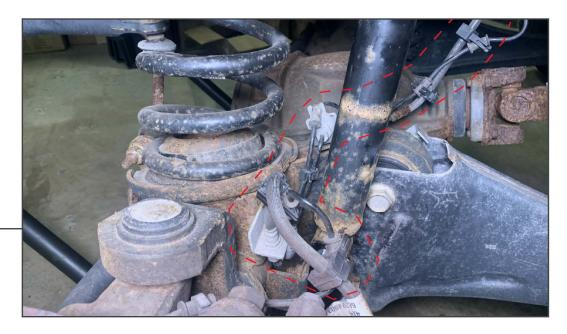
Secure the brake lines to the axle using the original (2) 13mm bolts. Massage the brake lines as necessary for best fit if necessary.
