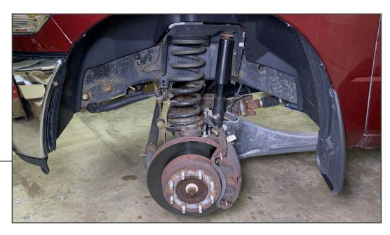
Safely lift and support the vehicle using a floor jack and jack stands. Remove the front wheels from the vehicle.
