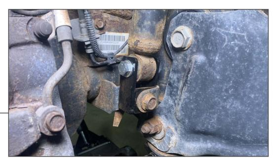
Twist the shock base 90 degrees, and secure the shock absorber into the previously mounted bracket using (1) M14 x 80mm bolt, (2) M14 flat washers, and (1) M14 lock nut. Tighten the shock until fully secure.
