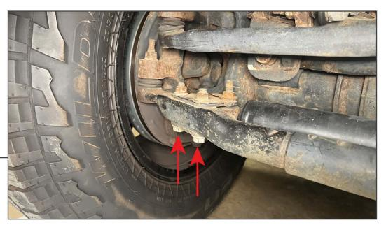
Locate the original vehicle steering stabilizer. Remove the steering stabilizer bracket from the tie rod by removing the (2) 18mm bolts/nuts, and use a pry bar to remove the mounting bracket and stabilizer from the tie rod.
