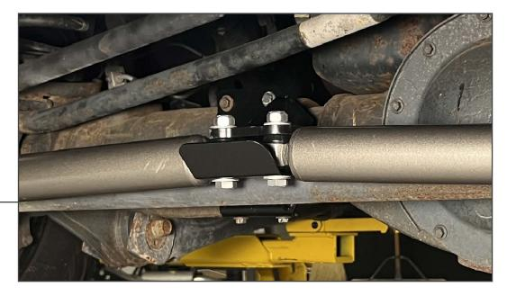
Fit each stabilizer shock to the center mounting bracket. Use the (1) axle clamp bracket under the stabilizer shocks, and secure into place using (1)  $1/2-13 \times 2.75$ " bolt, (2) 1/2" flat washers, and (1) 1/2" lock nut per stabilizer shock.
