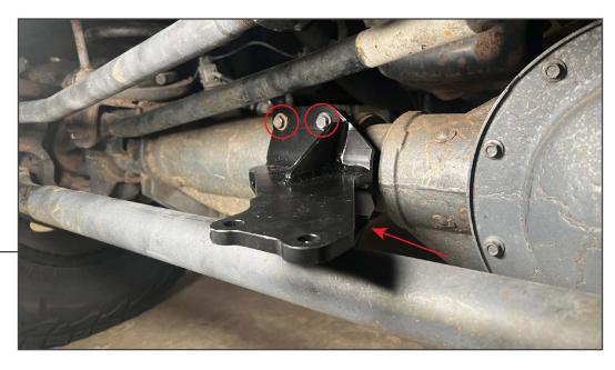
Fit and secure the included axle mounting bracket to the original steering stabilizer bracket mount on the axle tube using the original (4) 13mm bolts.
