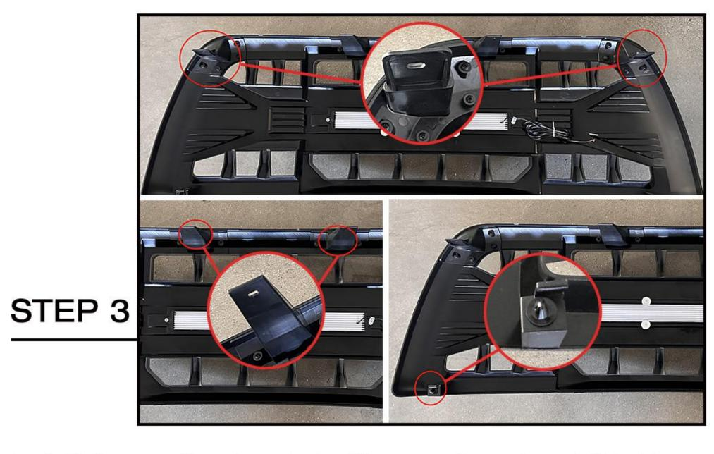
Install 4 mounting brackets.(2 on each end and 2 in the middle).Install 2 metal clips on each end.
