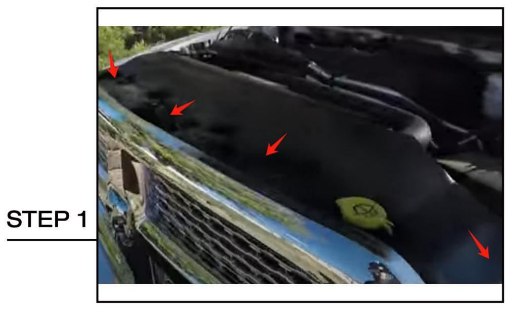
Open the hood, remove 4 plastic clips to remove shroud cover from vehicle.
