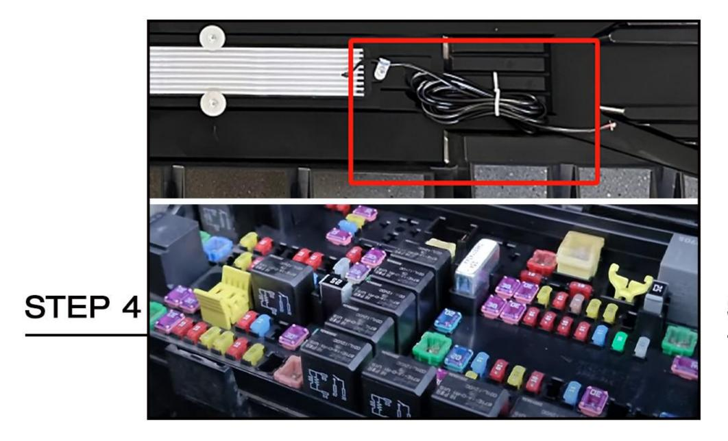
DRL Wiring: Wire to fuse box, the red wire connects to the ACC, the black wire connects to the negative of battery.
