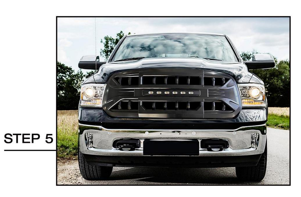
Line up the brackets on top. Press the bottom in place and start installing your hardware (follow the step 1-2 in reverse order.) to complete the grille installation.
