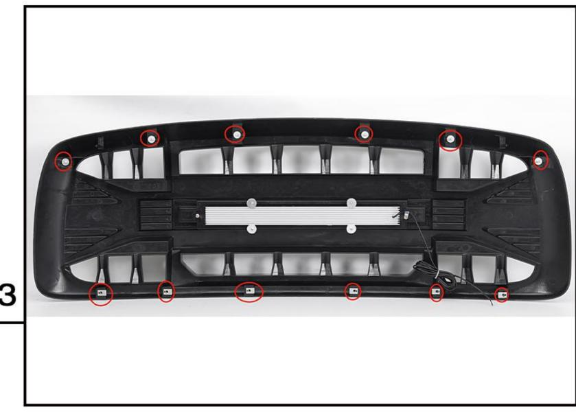
Open the hood, remove the six nuts on top, then put down the hood to pull the grille out of the car.
