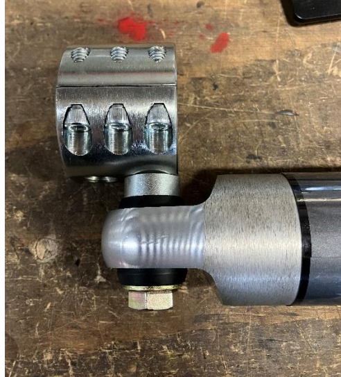
Figure 6. 4050-50 Clamp Installed on Steering Stabilizer.
