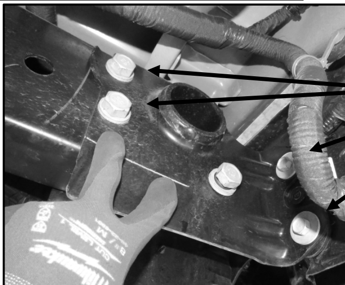
(Fig 2a) Starting at the rear DS remove the (4) OEM Hex Bolts
