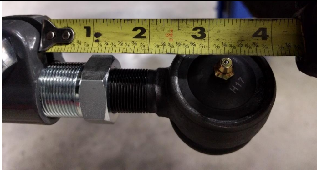
Figure 18. Tie Rod End Adjusted MAX 3.25" Out (Double Adjuster Side)
