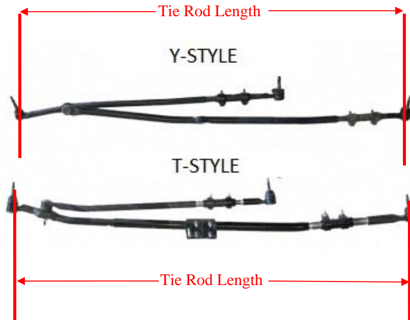
Figure 1. How to Measure Tie Rod Length
