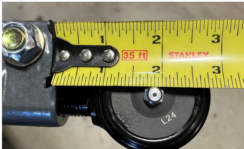
Figure 10. Passenger Side TRE Adjusted to 1 7/8" From the End of Tie Rod Forging.
