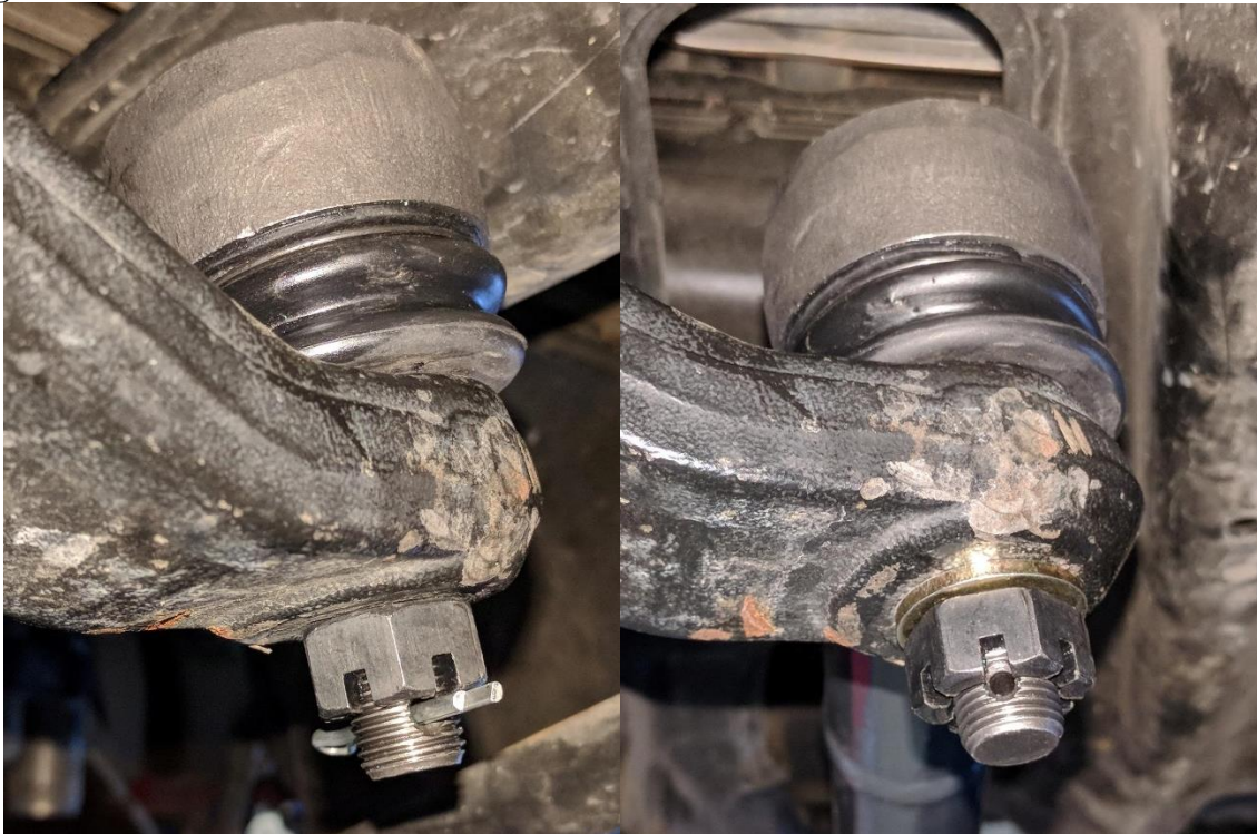
Figure 21 and 22. Washer Used Under Castle Nut
