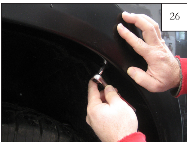
Hold flare in place while you start factory screws using an 8mm socket wrench. Do not tighten.
