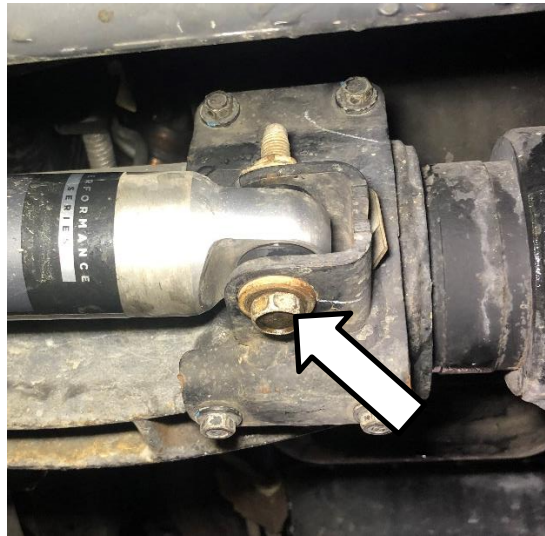
Figure 1. Stabilizer Bolt to be Removed
