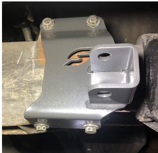
Figure 3. Loosely Installed Synergy MFG Stabilizer Relocation Bracket
