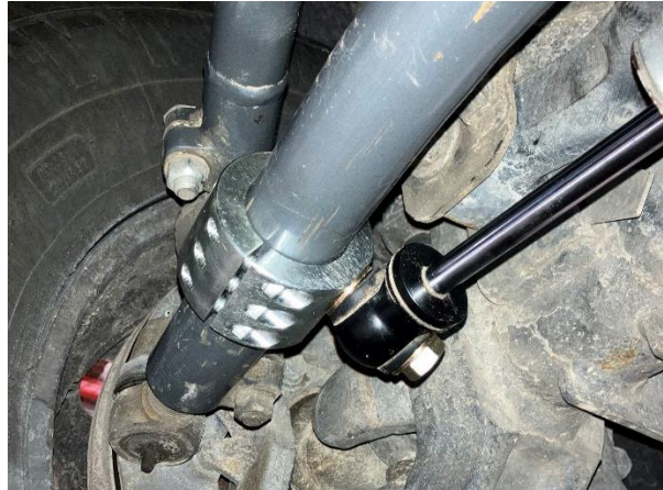
Figure 7. Installed Tie Rod Clamp and Steering Stabilizer
