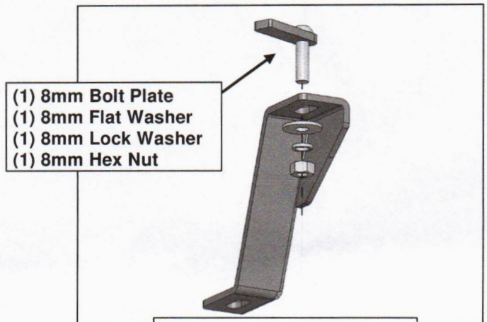
(Fig 5) Attach Skid Plate Mounting Bracket to Vehicle
