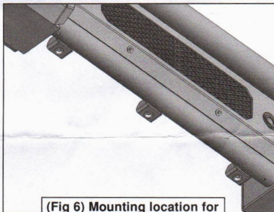
(Fig 4) Mounting location for Skid Plate Mounting Bracket on HD4 Bumper Mounting Bracket
