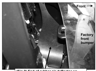
(Fig 2) End of rubber air deflector on driver side pictured from above bumper
