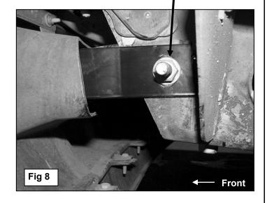
12mm x 45mm Hex Bolt (2) 12mm Flat Washers 12mm Lock Washer 12mm Hex Nut
