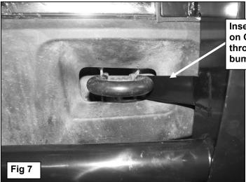
Insert mounting tab on Grille Guard through opening in bumper cover. Bolt mounting tabs on Grille
