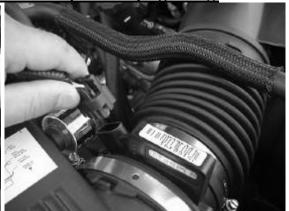
2. Remove Intake Hose and remove stock Mass Air Sensor
