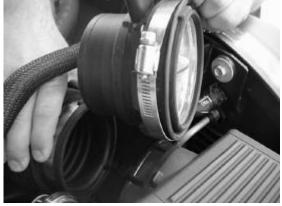
3.Remove gasket from stock Mass Air Sensor and install on Powr-Flo Sensor
