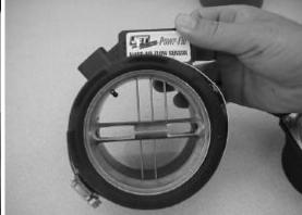
4.Install JET Powr-Flo Sensor, tighten all clamps and plug in harness
