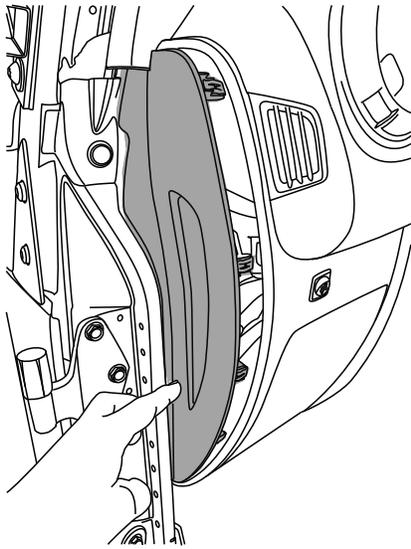
Reinstall all trim panels that were removed to install switch onto dash.
