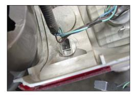
Reinstall the side marker light into the new housing. Connect the resistor box to the wire harness.
