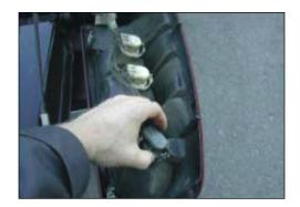
Remove the 4 bulbs socket from the stock lens. Remove the three bulbs leaving the side marker light installed.
