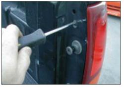
Open tailgate and remove the phillips head screws located inside the tail gate area.
