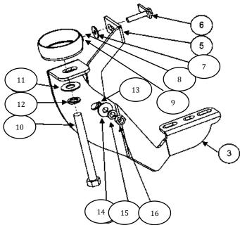
7. Install the middle bracket and attach with bolts before removed. Locates to the rubber plug that is in the rocker panel of the vehicle, remove and insert 5/16" bolt plate. Mounts the rear auxiliary bracket and attach with: 5/16" flat and lock washers, 5/16" hex nut. In the other side of the bracket attach with the rear bracket:  $3/8 \times 1$ " carriage head bolt, 3/8" flat and lock washers, 3/8" hex nut
