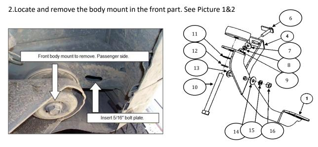
3. Install the front bracket and attach with bolts before removed. Locates the hole that is in the rocker panel of the vehicle and inserts 5/16" bolt plate. Mounts the front auxiliary bracket and attach with: 5/16" flat and lock washers, 5/16" hex nut. In the other side of the bracket attach with the front bracket:  $3/8 \times 1$ " carriage head bolt, 3/8" flat and lock washers, 3/8" hex nut.
