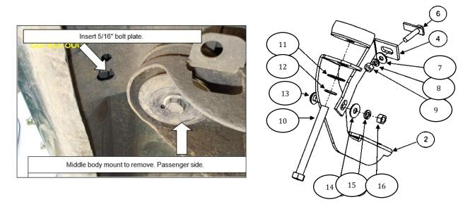
5. Install the middle bracket and attach with bolts before removed. Locates the hole that is in the rocker panel of the vehicle and inserts 5/16" bolt plate. Mounts the middle auxiliary bracket and attach with: 5/16" flat and lock washers, 5/16" hex nut. In the other side of the bracket attach with the middle bracket: 3/8 x 1" carriage head bolt, 3/8" flat and lock washers, 3/8" hex nut..
