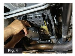
5. Double check the M6 Flat Head Screws (J) securing the Filter Support Pads (I) is tight. Install the Flat Gasket (B) or reuse the factory transmission gasket, then attach the Transmission Pan (A) using the supplied M6 Screws (G) and M6 Washers (H). Torque the bolts to 8-10 lb-ft following the crossing-pattern sequence shown below.
