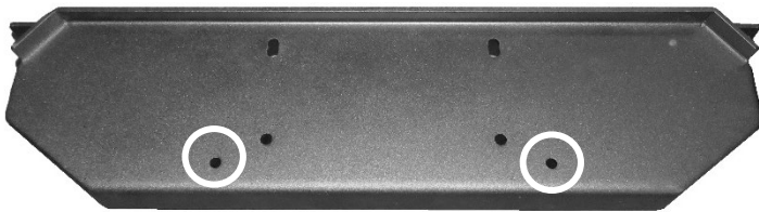
(Fig 1) Locate mounting holes on Winch Tray.
