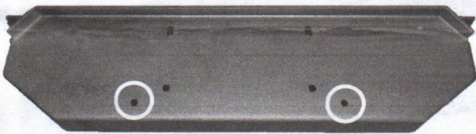
(Fig 1) Locate mounting holes on Winch Tray.
