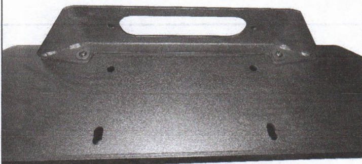
(Fig 3) Attached Fairlead Mount to Winch Tray.
