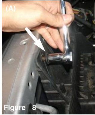
Figure 6 (A) Use a 8mm nut driver and loosen clamp on air duct connected to throttlebody. Figure (B) Pull air duct off of throttlebody
