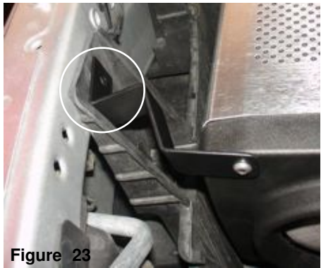
Figure 22 Install the bracket p/n:x-20109 to the power-flow box. Make sure its install to the back side of the power flow box. Install grommet to the bracket hole.
