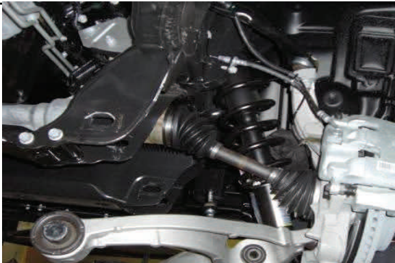
Remove strut assembly from vehicle.
