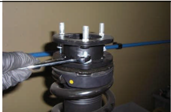
Attach new strut extension with OE hardware.
