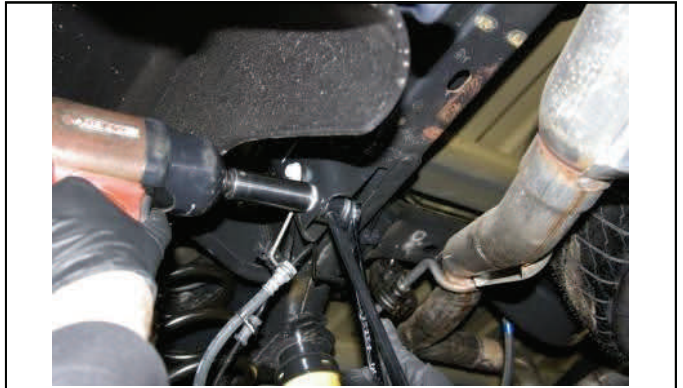
Disconnect upper sway bar end links.
