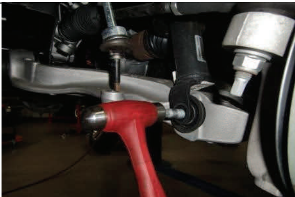
Gently tap lower strut mounting bolt out.
