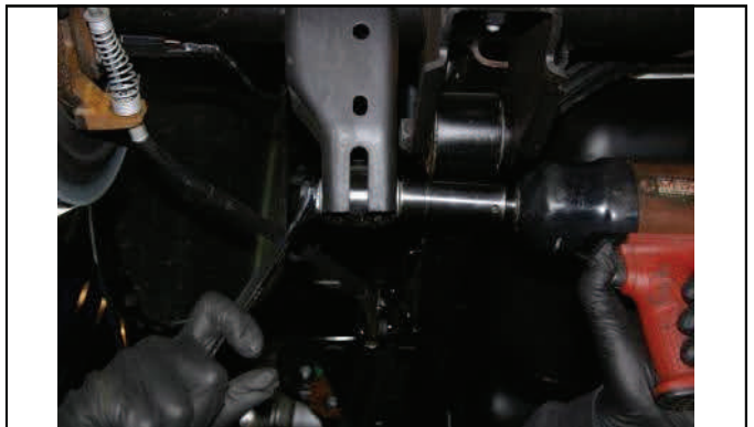
Remove lower shock mounting hardware.
