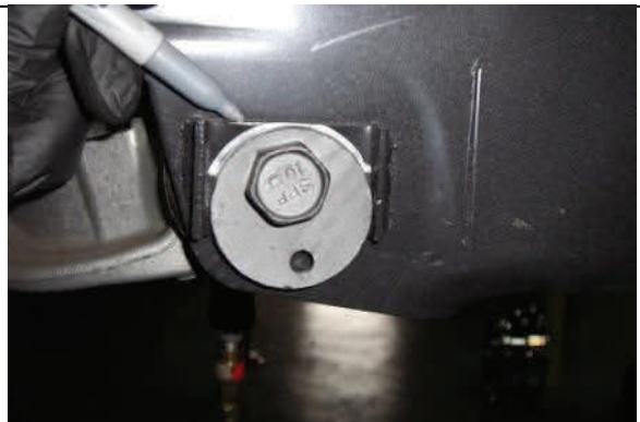
Mark front and rear lower control arm alignment cams.
