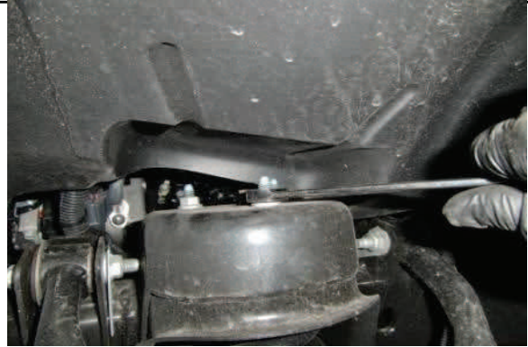
Now, remove upper strut mounting nuts.
