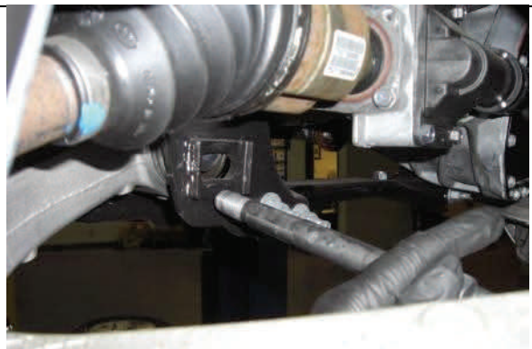
Remove lower control arm mounting bolts.
