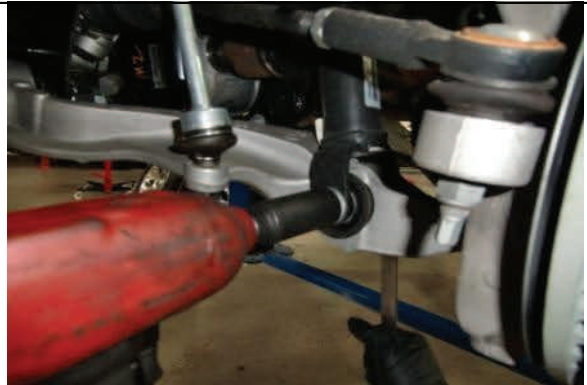
Remove lower strut mounting nut.
