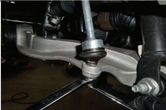
Remove lower sway bar end link at control arm.
