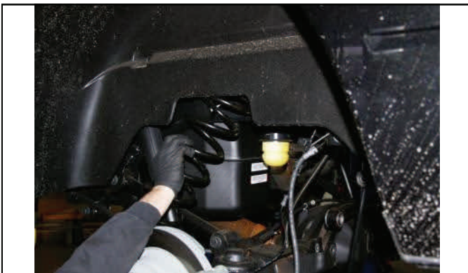
Carefully lower axle, remove spring and upper rubber isolator
