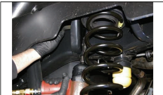
Reinstall OE isolator and coil spring, raise suspension.
