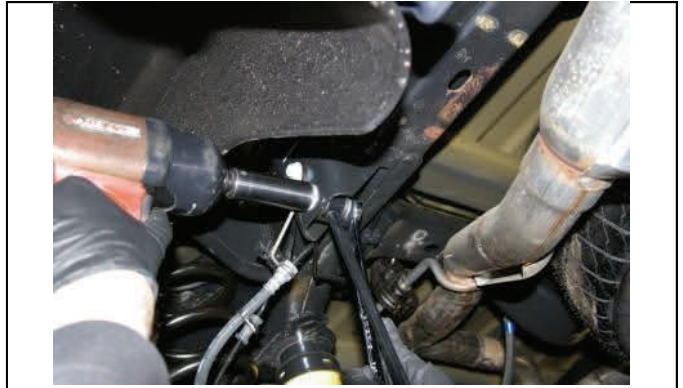
Disconnect upper sway bar end links.
