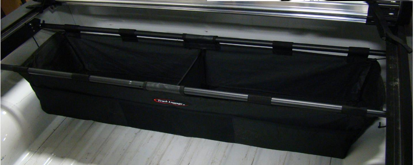
NOTE: Place driver and passenger brackets the same distance from the front bulkhead
