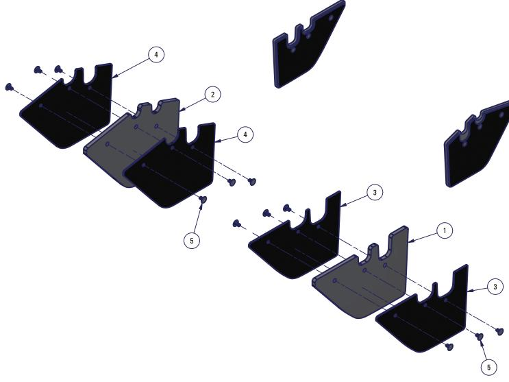
Step 1: Use the provided hardware to assemble the gun rack \ dividers. Place a stiffener on each side of the foam and line up the holes.
