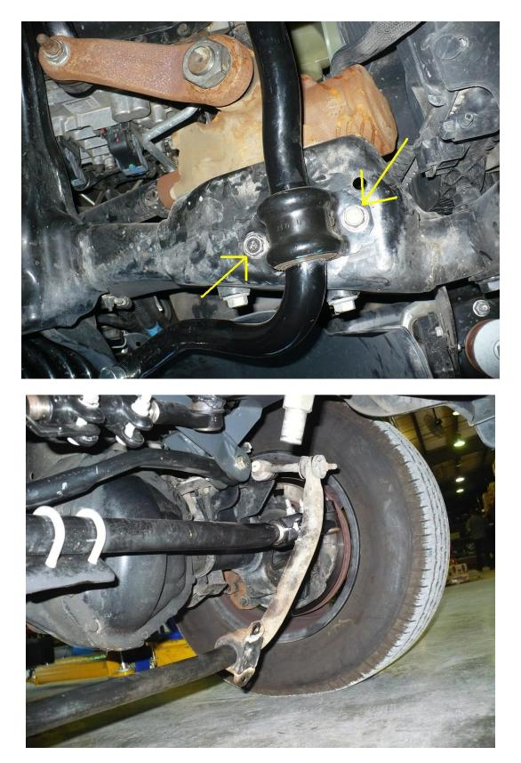
2) Next remove the pitman arm nut on the steering box and install the Pitman arm stud provided in the kit along with the new lock washer provided. Torque to 185 ft-lbs.
