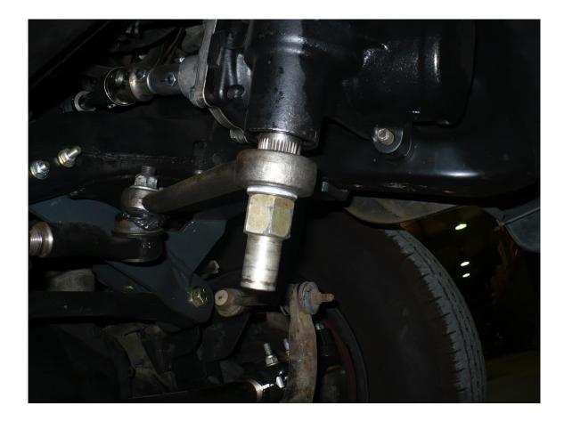
3) Next, position steering box brace onto sway bar as shown and swing into place. *NOTE*; 8557-04 shown in this installation. Parts will differ slightly on 8558 & 8559 kits, but installation is the same. Start the M10-1.50 bolts into the threaded holes on the frame. Use a large flat washer and lock washer under the head of the bolt.
