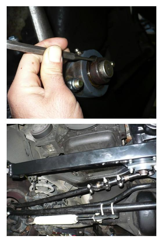
8) Recheck bolts / torques after 100 miles of driving. Grease bearing at normal chassis service intervals.
