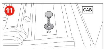
Insert the large flat bolt with the supplied rubber washer through the front panel and silver slotted bracket underneath. Repeat on other side.
