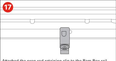
Attached the prop rod retaining clip to the Ram Box rail where it will meet the prop rod when rotated down.
