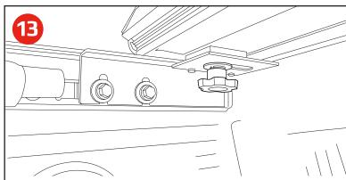
Mount cover with elevator bolt, rubber washer, flat washer, lock washer and star knob in order. Center cover in the bed opening and tighten.
