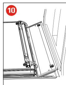
The small panel faces forward, toward the cab and folds down over the silver brackets. The front panel must sit just inside the bulkhead rail with the seal resting on top of the rail. Fold the panel down and align it so it is setting squarely on the rails and align the mounting holes with the silver slotted brackets on the rails.
