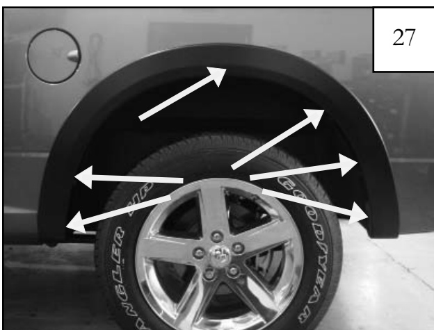
Supplied screw locations. Install one supplied screw at the top of flare first for easier installation. See step 28.
