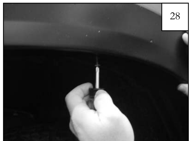
Start #8x3/4" Washer Panhead Screws using a Phillips screwdriver. Do not tighten. Pictured here is the top center screw location of the rear wheel well.
