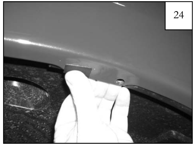
Install plastic tab over existing factory hole.
