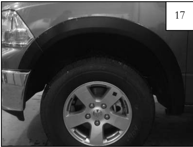
METAL BUMPER ONLY: Completed front flare installation.
