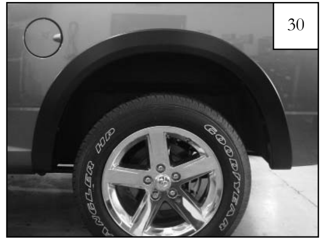
Completed rear flare installation.
