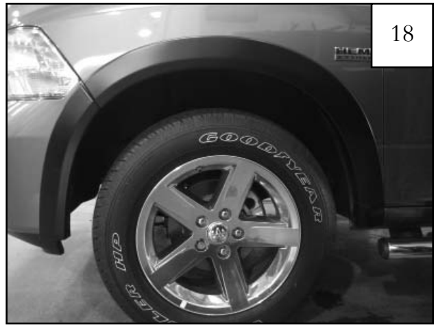
PLASTIC BUMPER ONLY: Completed front flare installation.
