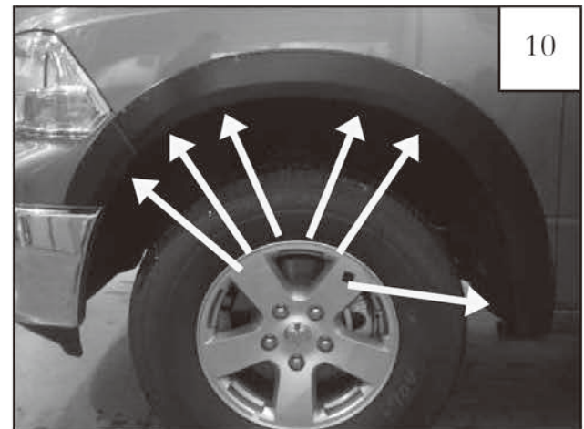
METAL BUMPER ONLY: Press firmly on flare and tighten all screws.
