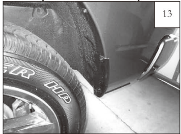
2013-Up Models Only : You will need to remove the plastic factory wheel well piece from the rear of the wheel well. Please follow steps 21 - 22.
