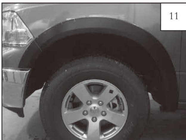
METAL BUMPER ONLY: Completed front flare installation.
