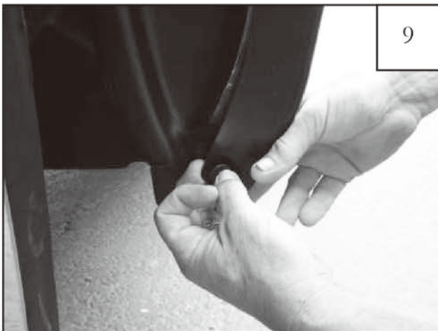
Slide factory screw through hole in flare, and start factory screw with an 8 mm socket wrench. Do not tighten
