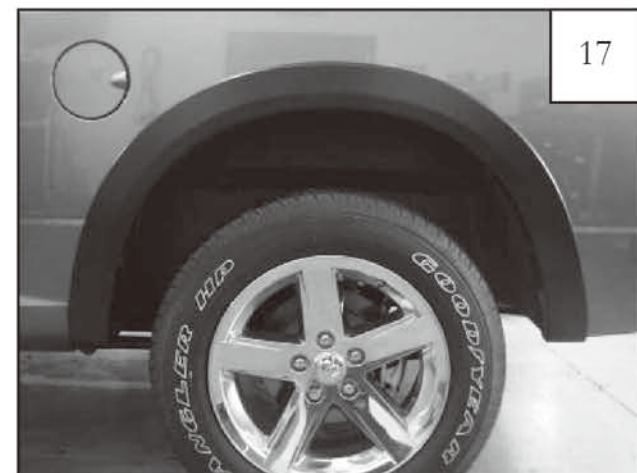
Completed rear flare installation.
