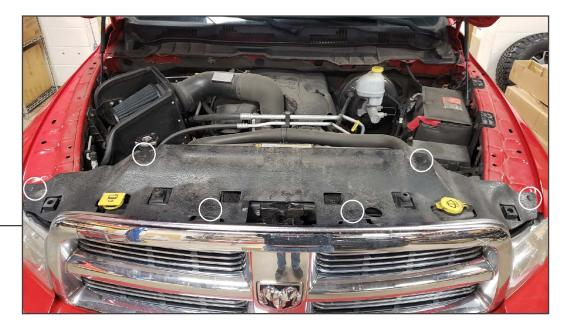
Open the hood. Using a plastic prying tool, locate and remove the (6) push clips securing the radiator cover to the vehicle. Remove radiator cover from the vehicle.
