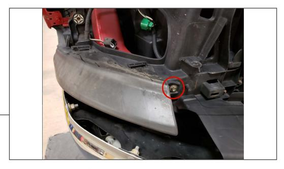
Located under the headlight, remove the (1) 10mm bolt on each side securing the bumper cover supports to the vehicle. Remove the supports.
