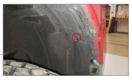
Located on the front wheel well liner, using a trim panel removal tool remove the (1) plastic push clip to gain access to the headlight retaining clip.
