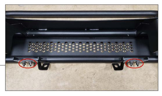
Install the (2) inner mid plate brackets with the optional (2) grille lightbar brackets. Each side use (2) M8x30mm allen bolts, (4) flat washers, (2) lock washers, and (2) nuts.
