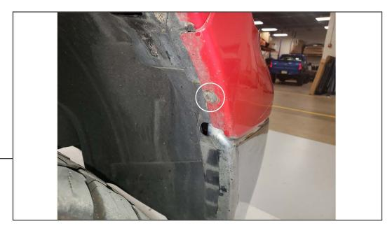
Using a 7mm socket & ratchet remove the screw securing the bumper cover to the fender liner. Then using a trim panel removal tool, remove the (2) plastic push clips. Repeat for the opposite side.
