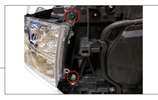
Locate, and remove the (2) 10mm bolts securing the headlight to the front support. Gently pull the headlight away from the vehicle. Unplug the headlight wire connectors, and remove the headlight from the vehicle.
