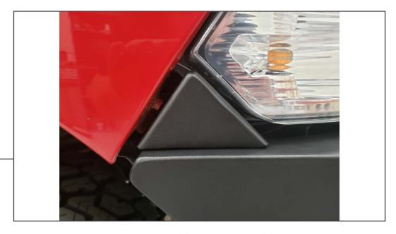
Install the headlight filler triangles each side will use (2) M6 Allen Bolts, (2) M6 Lock Washers, and (2) Flat Washers.
