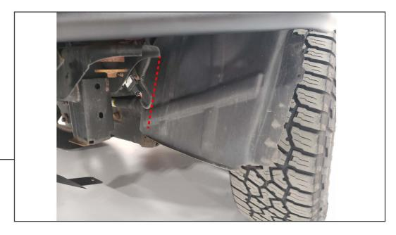
Trim, cut, or remove the exposed portion of the fender liner to prevent it from rubbing on the tire.
