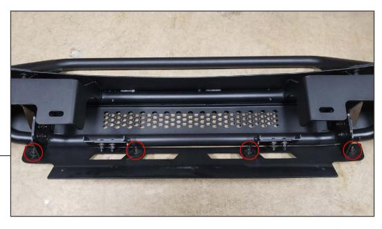
Install the mid plate to the bumper using the (4) M8x30mm allen bolts, (8) flat washers, (4) lock washers, and (4) nuts.
