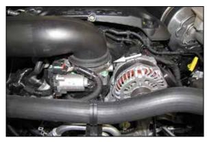
3. Loosen the hose clamp at the throttle body and then lift the complete intake system out of the vehicle.
