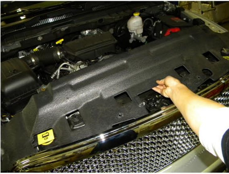
23. Replace the plastic guard
