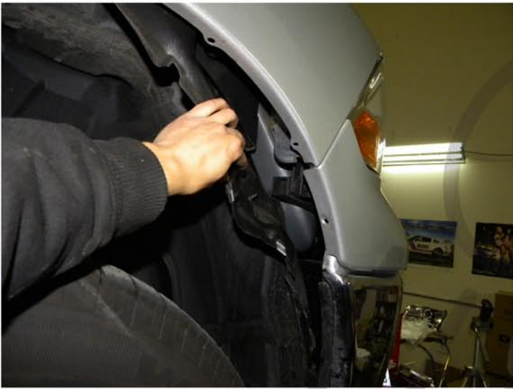
25. Pull the liner to the side
