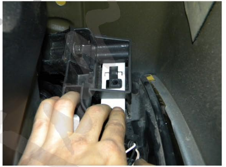
26. Lock the plastic headlight retainer
