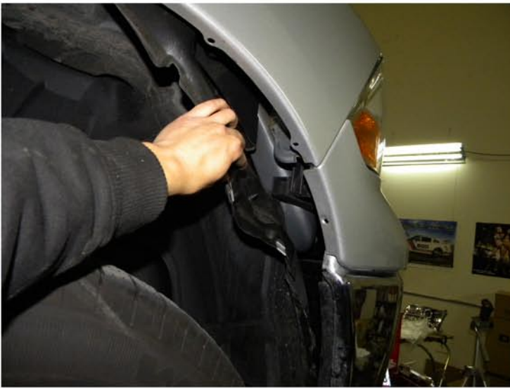
11. Pull the liner to the side
