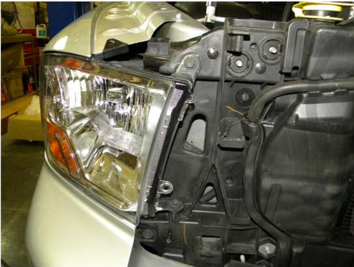
7. (2) 10mm bolts location
