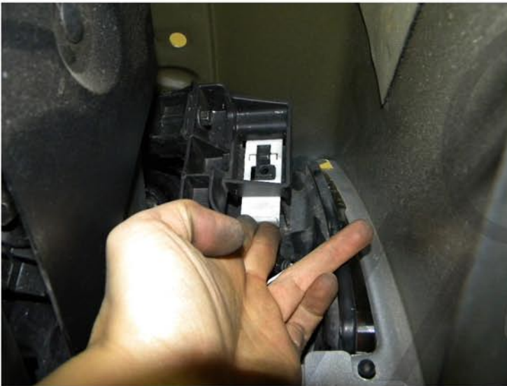
13. Push the retainer up to unlock the headlight
