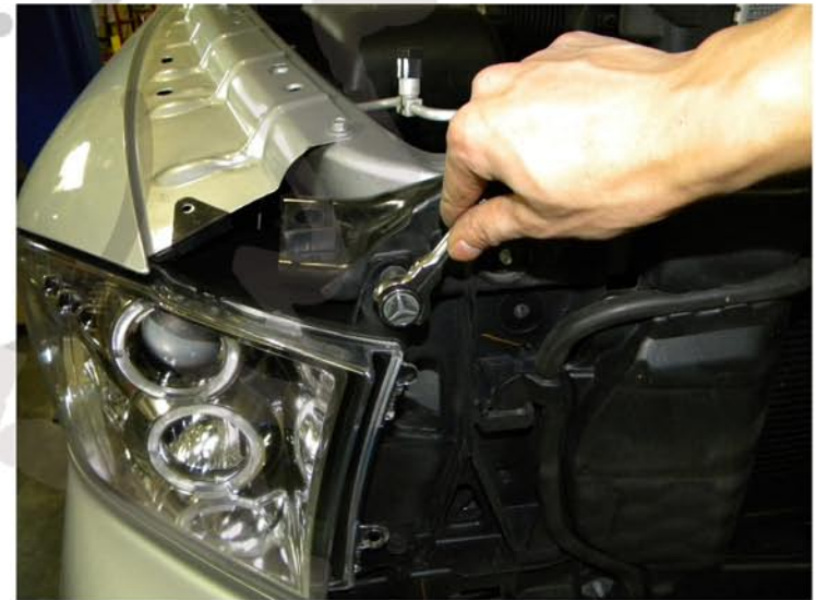
20. Tighten the (2) 10mm bolts
