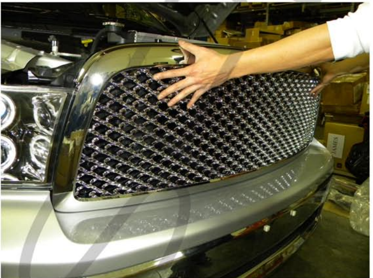
21. Replace the front grill
