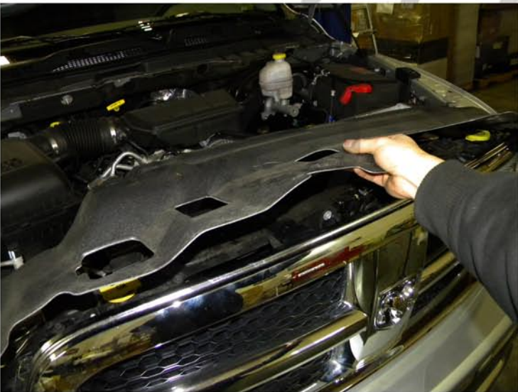
3. Remove the plastic guard
