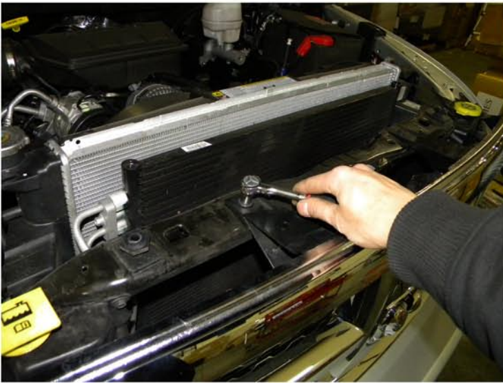
5. Remove the (4) 10mm bolts
