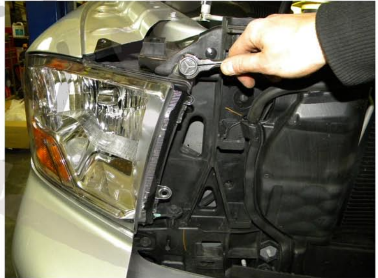
8. Remove the (2) 10mm bolts
