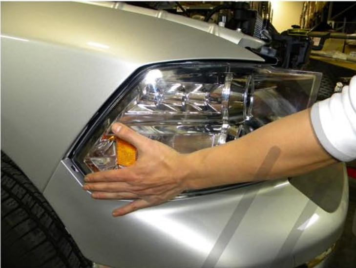
19. Place new headlight in the stock location
