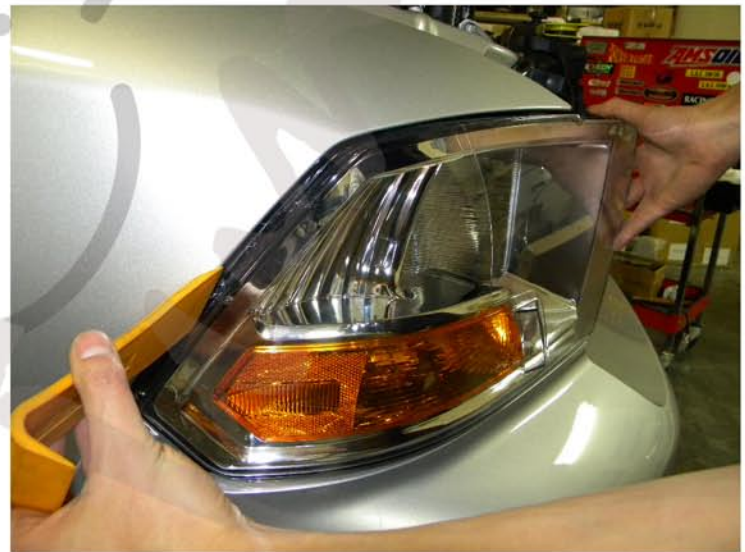
14. Remove the headlight
