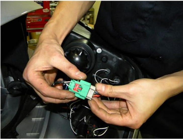
17. Connect the headlight harness into the new headlight Please see the Halo and L.E.D installation instruction If your headlights don't have HALO or L.E.D. You can skip it
