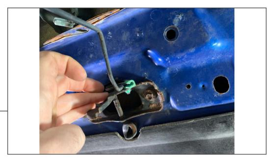
Begin by opening the hood to gain access to the backside of the factory grille. Unclip the hood latch release from the hood latch. Remove the hood latch release rod from the grille.
