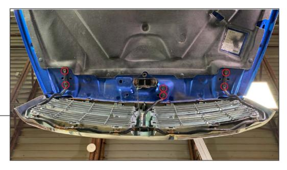
Using the same 8mm socket, remove the (6) bolts securing the grille brace to the underside of the hood.
