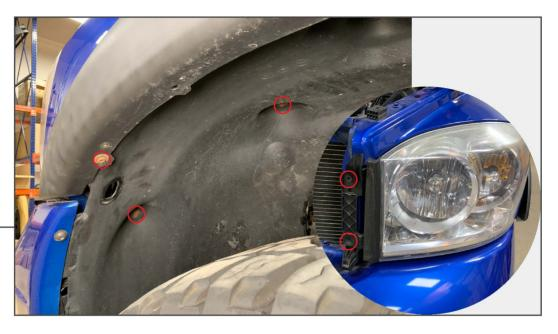
Remove the (3) 8mm screws securing the fender liner to the vehicle. Fold back the fender liner to access the nut securing the headlight to the vehicle. Then, remove the (2) 10mm bolts from the front of the headlight. Pull the headlight away from the vehicle.
