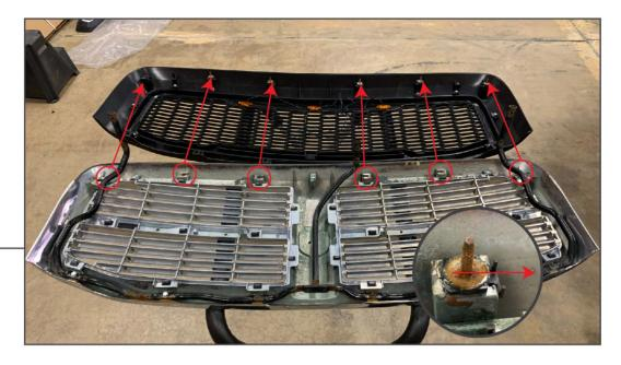
Transfer the (6) clip stud fasteners across the top of the grille onto the new grille.
