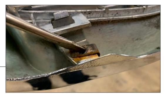
Transfer the (6) clip nuts from the factory grille onto the new grille.
