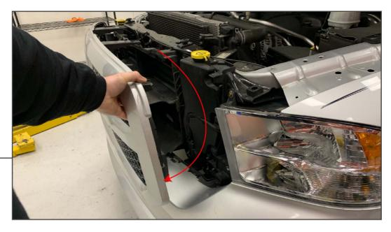
Place your hand down behind the grille and press at the bottom of the grille away from the radiator support and pull the grille away from the vehicle.
