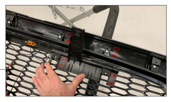
Align the supplied center brackets to the back of the grille. Each bracket has a specific location on the grille. Line the alignment tabs up with each bracket. Then attach the brackets to the grille using the supplied screws.
