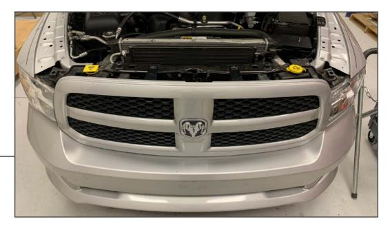
Remove the air dam across the top of the radiator support. Using a soft pry tool, remove the plastic push clips securing the air dam to the vehicle.
