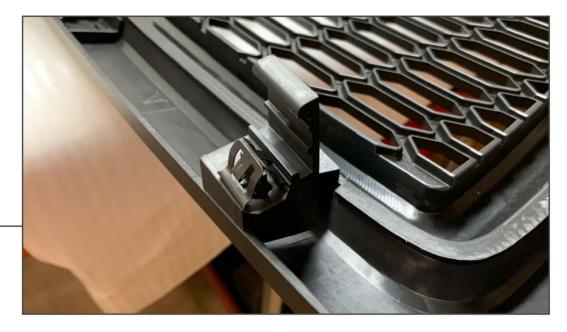
Press the suppled push clips into the (2) lower grille clip locations.
