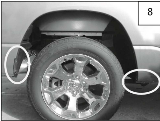
Locate the (2) factory installed mud flaps on the passenger side rear wheel well.
