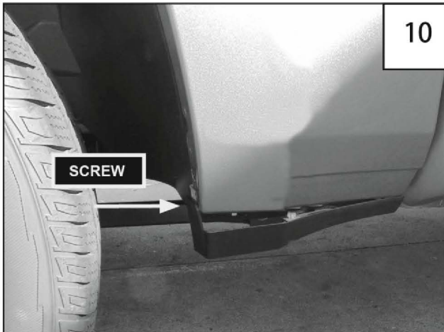
Remove and keep (1) factory installed screw, and remove mud flap from vehicle. This factory screw will be used to install the rear fender flare.
