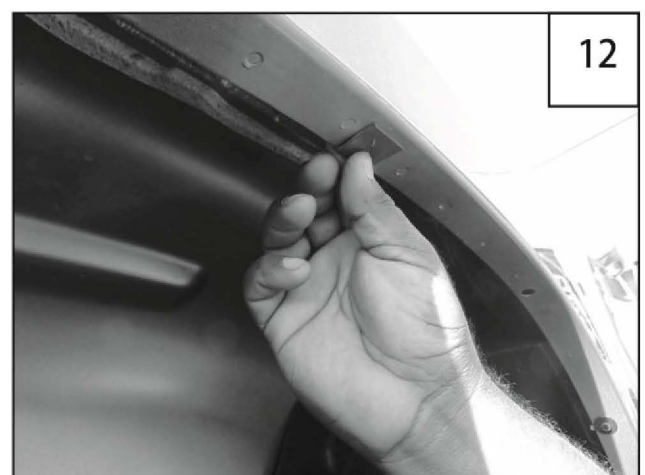
Install supplied Tab (MT1-0014) over existing factory hole.
