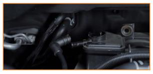
Release the tab on the clip that holds the PCV hose. Then remove the hose from the engine bay.
