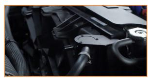
12. Connect the shorter hose to the outlet port on the catch can. (1x worm gear clamp)
