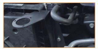
8. Install the additional bracket piece to the back of the catch can bracket. (1x 10mm bolt)
