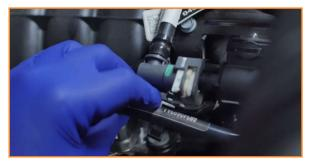
Feed the longer hose under the intake and connect it to the PCV valve housing. (1x worm gear clamp)
