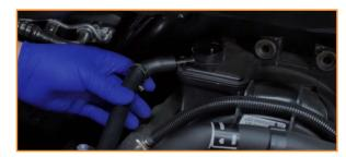
5. Install the smaller hose to the intake port. (1x worm gear clamp)
