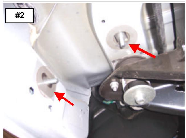
**STEP-3** ATTACH THE DRIVER SIDE FRONT BRACKET TO THE BODY PANEL USING THE T-PLATE (2) 3/8" X 1/4" HEX BOLTS, (3) 3/8" FLAT WASHERS, (3) 3/8" LOCK WASHERS AND (1) 3/8" HEX NUT. HAND TIGHTEN. **PHOTO #3**
