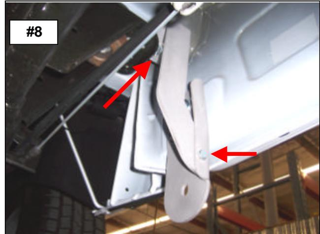
**STEP-9** ATTACH THE DRIVER SIDE STEP TO THE FRONT AND REAR BRACKETS USING (1) 1/2" X 2" HEX BOLT, (1) 1/2" FLAT WASHER AND (1) 1/2" LOCK WASHER FOR EACH BRACKET.
