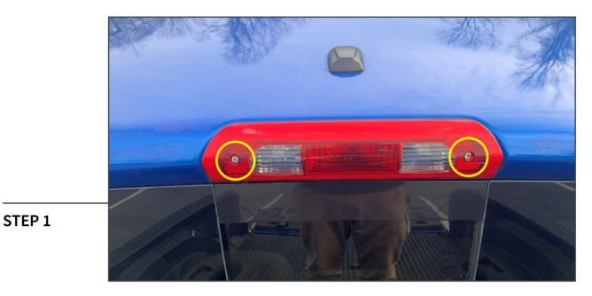
Remove (2) Phillips head screws from the third brake light assembly.
