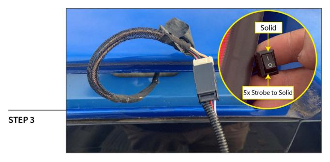
Plug in the brake light electrical connector into the vehicle's wiring harness. Toggle the switch to enable 5x strobe feature.
