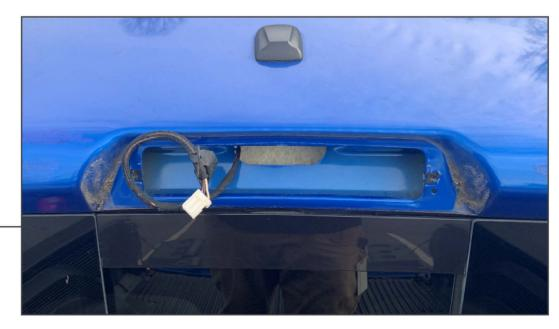
With the screws removed, remove the brake light from the vehicle using a plastic pry tool. Unplug the electrical connector from behind the brake light.
