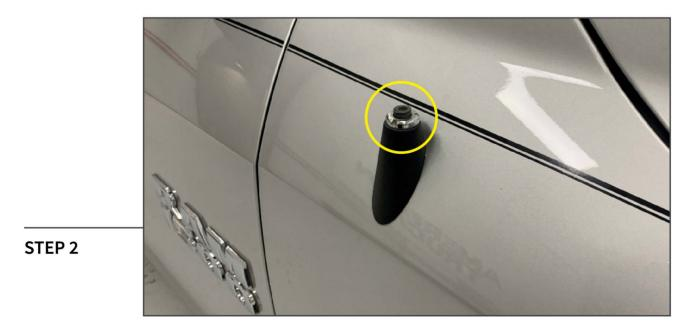
Using pliers or channel locks, loosen the nut at the top of the antenna base. Un-thread the nut entirely and set aside. The nut will be reused for assembly.
