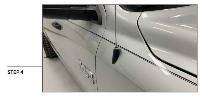
Install the new antenna base to the vehicle following steps 1-3 in reverse order.
