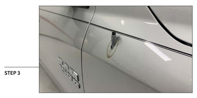
Lift the antenna base cover from the vehicle. Clean any dirt and debris previously captured by the antenna base from the vehicle using exterior detailer and a microfiber cloth.
