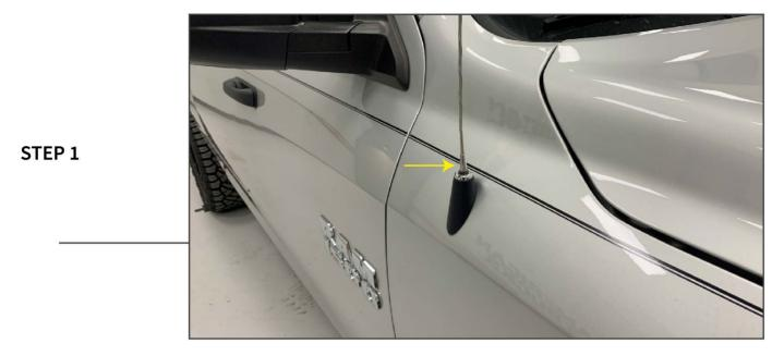
Using an adjustable wrench, loosen and remove the antenna from the vehicle.
